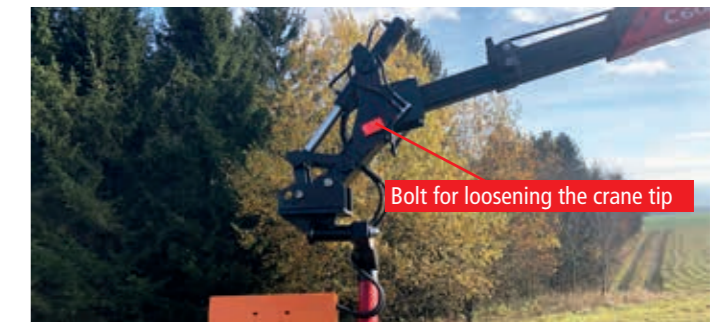
Kotschenreuther "Shoe" changing system for crane tip, hydraulically adjustable kinematics for attachment of e.g. pruning shears.
