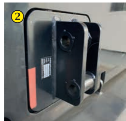
2 Rotatable hitch adapter in the back wall - in minutes you can attach your trailer to the back wall.
