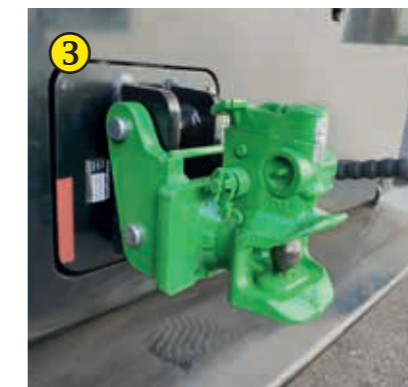
3 Tow hitch on swivel adapter attached to the rear panel, with StVZO approval.
